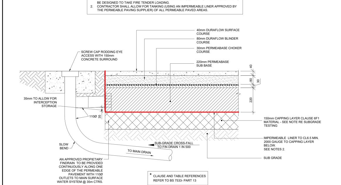
DETAILED DESIGN OF THE PAVEMENT BUILD-UP, THE FIN DRAIN LAYOUT & FIN DRAIN OUTLET LOCATIONS BY THE SUPPLIER IN ACCORDANCE WITH BS7533-PART 13. THE PAVEMENT IS TO
